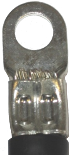
Close up of “M” Profile Crimp
